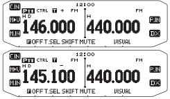
If you are using an E type transceiver, when operating on the 430 MHz band, the offset direction changes as follows:
