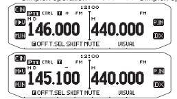
If you are using an E type transceiver, when operating on the 430 MHz band, the offset direction changes as follows:
