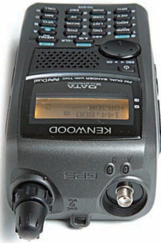
The very simple plain top with the recessed SMA antenna connection.
