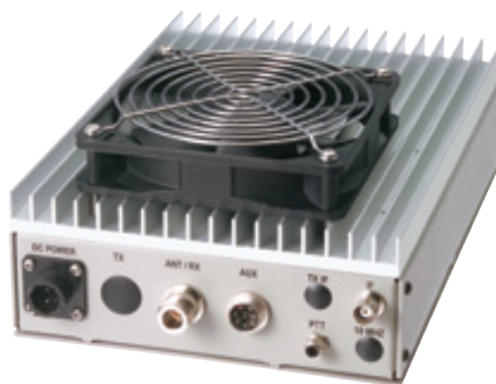
Figure 5 — The rear panel of the L222-28 features an AUX connector with all control signals so that no additional connectors are required if the configuration is changed.
