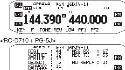
When a duplicate message from the same station is received, an error beep sounds; however, an acknowledgment is returned. "dM" and a call sign appear on the display.
