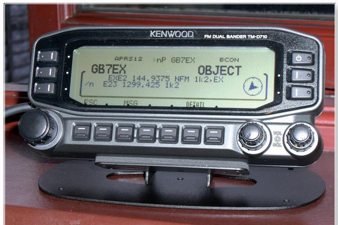
*Fig. 3: The '710E acts as a stand-alone Packet Radio unit.*
