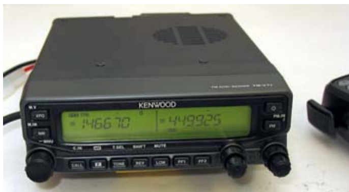
Kenwood TM-V71A 144/440 MHz transceiver.
